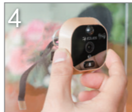
4 Fasten the camera by pressing it firmly onto the door.
