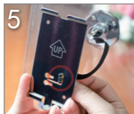
5 Hold the bracket upright(see the UP arrow on the bracket),slide the ribbon cable through the middle slot on the bracket.
