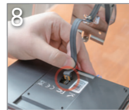
8 Plug the ribbon cable into the port on the back of the screen.
