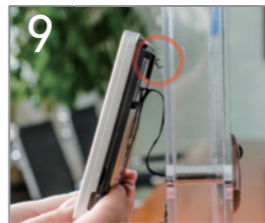
9 Hang the screen with the concave on its back aligning with the top of the bracket.
