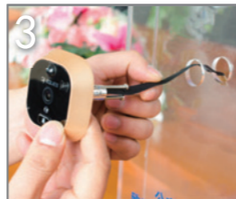
3 Pass the ribbon cable through the door hole.
