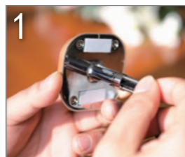
1 Attach two bolts to the camera loosely.
