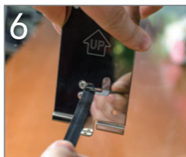
6 Align the round end of the top and bottom slots on the bracket with the two bolts on the camera, then slide the bracket toward the camera.
