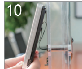
10 Swing the lower screen toward the lower bracket.The strong magnet will hold two parts together firmly.
